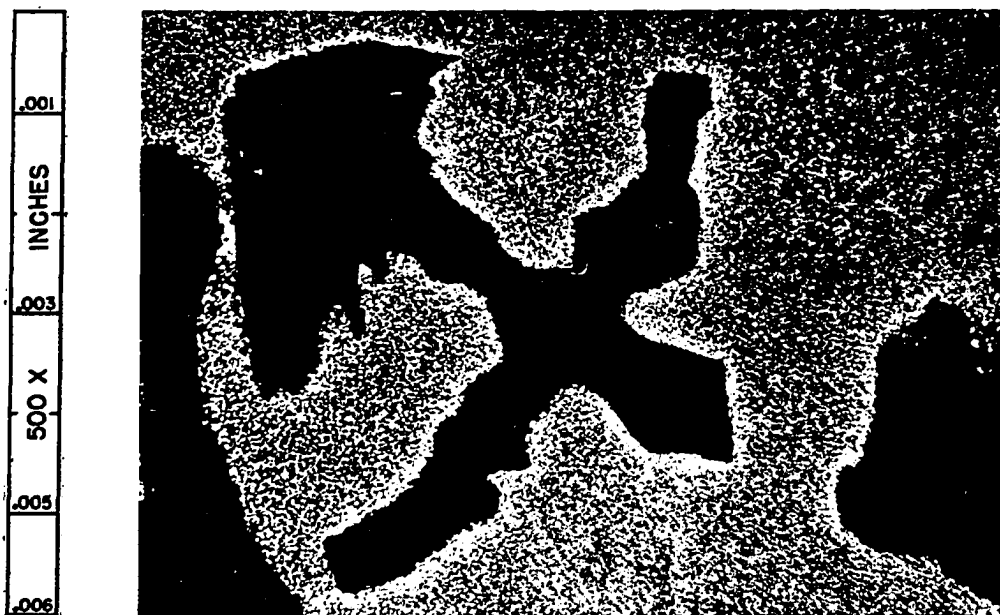
Figure 13. Photomicrograph showing cadmium molybdate ( \text{CdMoO}_4 ) precipitate in cadmium after testing in molybdenum for 300 hours at 700°C. Cadmium initially contained 1000 parts per million oxygen in the form of \text{CdO} . Sample Number 170 (500X)
